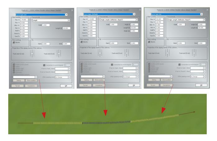
To my first line rail, I add a second clothoid rail with a start angle of 0° and an end angle of 5°.
